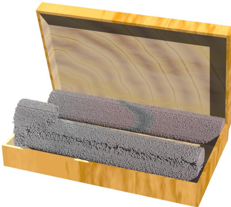
Fig. 9 Simulation of deformation of cylindrical sample of mudstone taken by boring exploration in core box. Magnification ratio of the figure is 1.0
