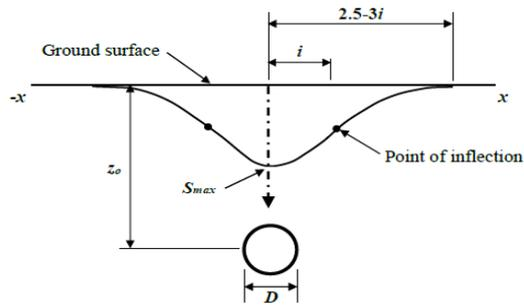
Fig.3 Definition of settlement trough of Gaussian form
