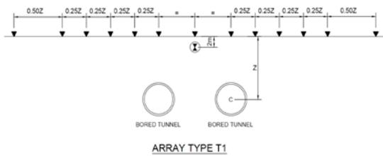
Fig.4 Typical array of surface settlement monitoring
