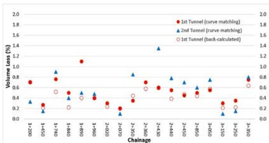
Fig.8 Back-analysed volume loss in Kenny Hill Formation by EPB TBM
