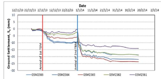
Fig.6 Typical surface settlement trends when TBM passed through
