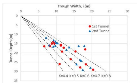
Fig.10 Values of trough width parameter obtained from curve matching
