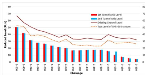
Fig.5 Anticipated ground conditions and tunnel depth at selected monitoring arrays
