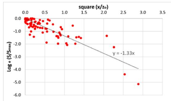
Fig.9 Back-calculated trough width parameter
