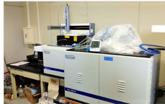
Fig.5 Isotopic ratio measurement system (Sercon Geo Wet System)
