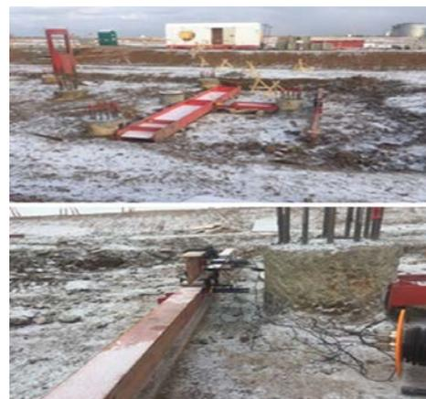
Fig. 6 Static Lateral Pile Loading Test in construction site Aksay
