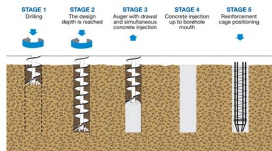
Fig. 1 The CFA construction sequence
