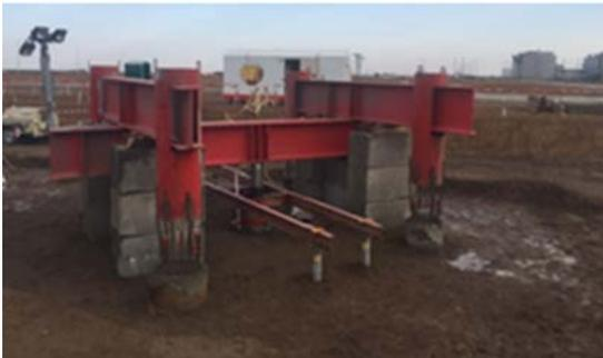
Fig. 2 Field pile test by SCPLT method
