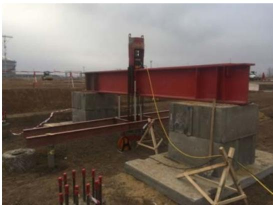
Fig. 4 Static Tension Pile Loading Test in construction site Aksay
