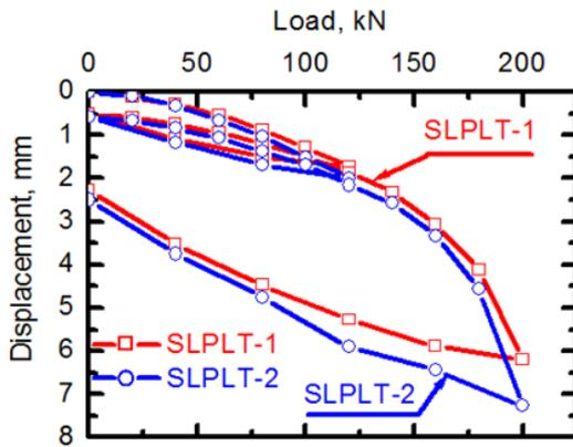
Fig.7 Results of Static Lateral Pile Load Test (SLPLT-1 and SLPLT-2)
