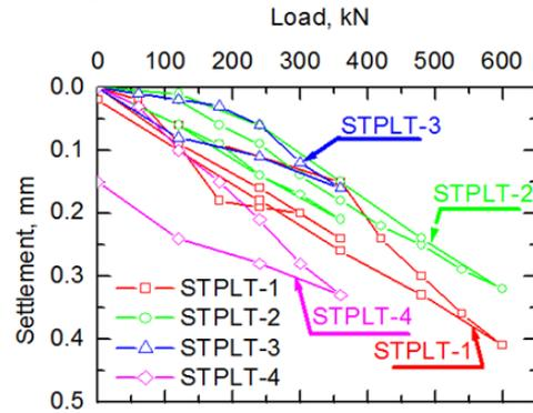
Fig. 5 Results of Static Tension Pile Load Test of piles SCPLT (1, 2, 3, 4)
