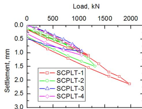
Fig. 3 Results of Static Compression Pile Load Test of piles SCPLT (1, 2, 3, 4)
