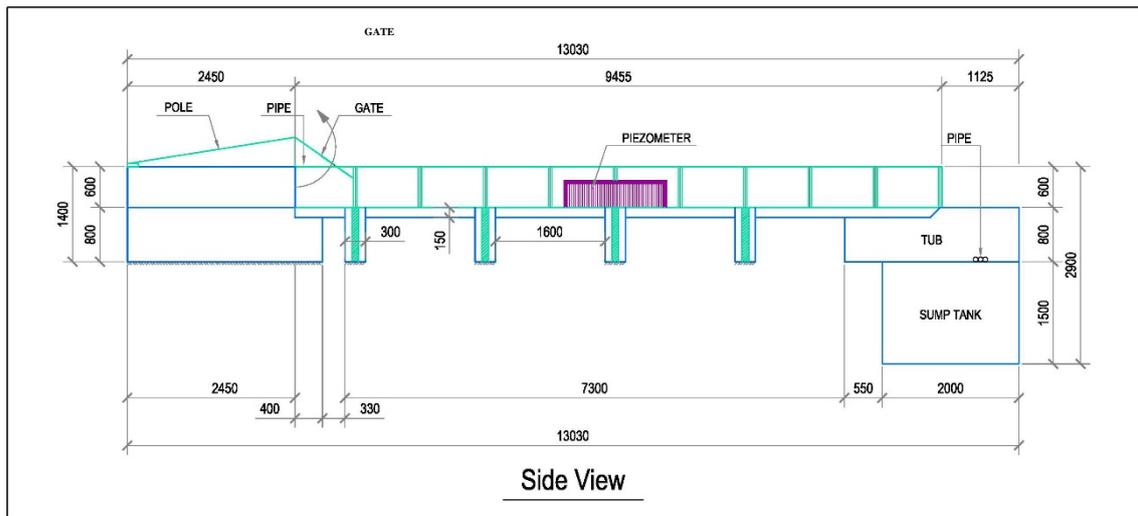
Fig.1b Layout of the constructed physical model (side view)
