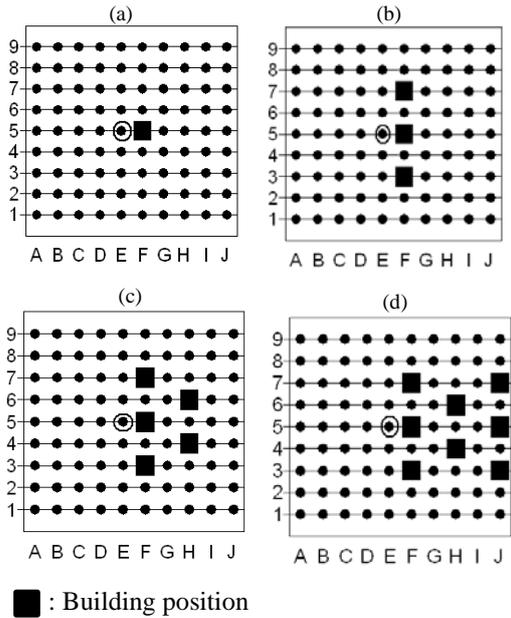
Fig.4 Configurations of blockages: (a) one building, (b) three buildings, (c) five buildings, and (d) eight buildings
