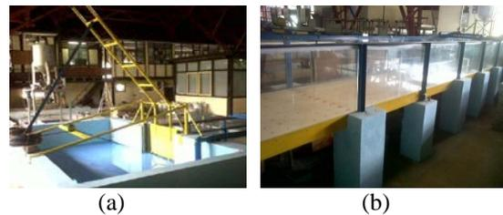
Fig.2 Dam break experimental model (a) Reservoir (b) Channel
