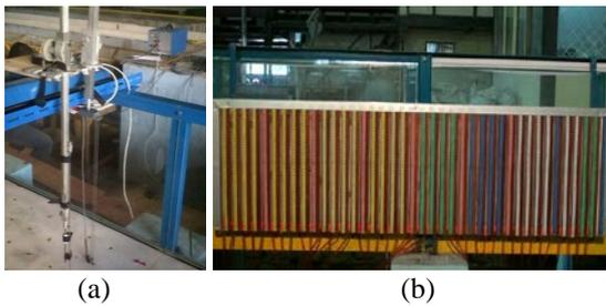
Fig.5 (a) Current meter and wave probe (b) Piezometer
