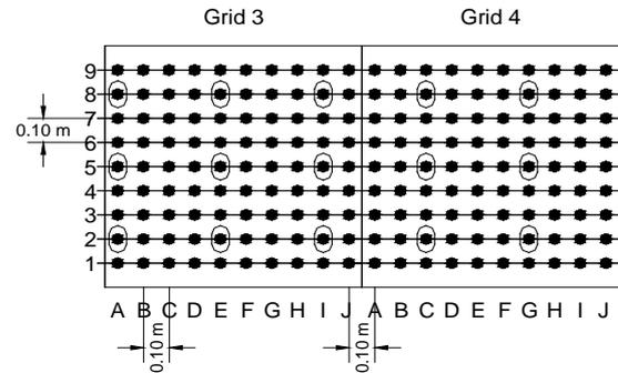
Fig.9 Position of flow velocity measurement for no building case
