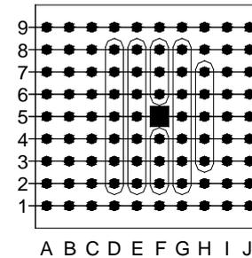
Fig.10 Position of flow velocity measurement for one building configuration
