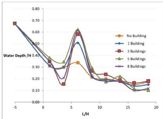
Fig.8 Comparison of water depth in long section profile for  $t = 5$  second and initial reservoir depth = 40 cm
