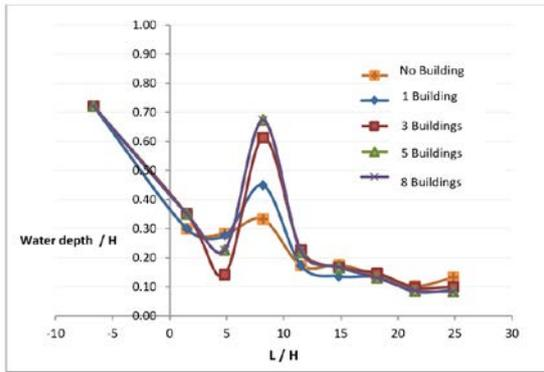
Fig.7 Comparison of water depth in long section profile for  $t = 5$  second and initial reservoir depth = 30 cm
