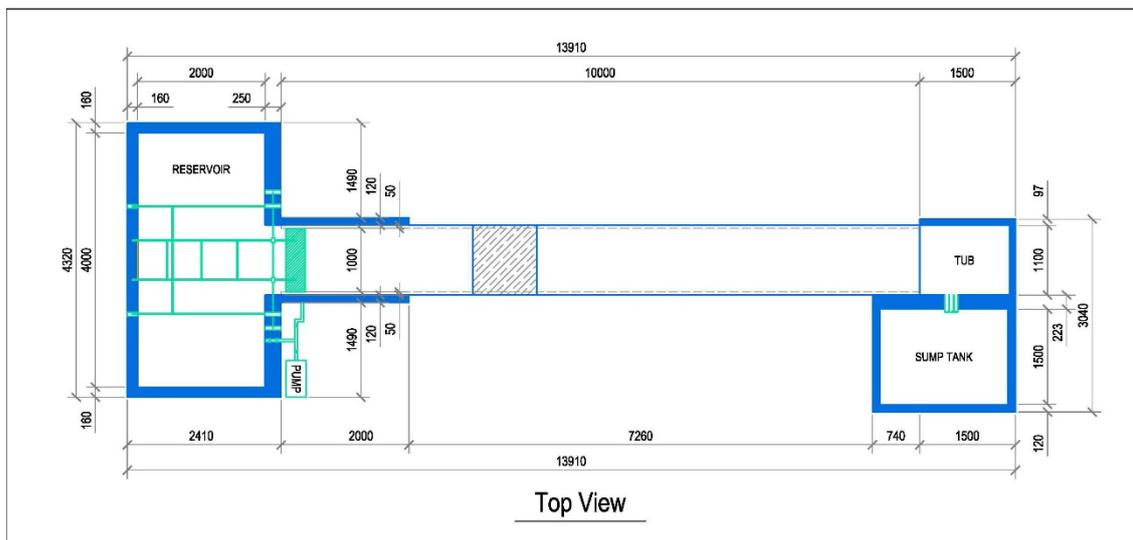
Fig.1a Layout of the constructed physical model (top view)
