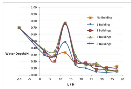
Fig.6 Comparison of water depth in long section profile for  $t = 5$  second and initial reservoir depth = 20 cm
