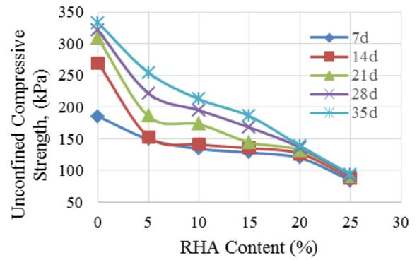
Fig. 7. Unconfined Compressive Strength vs RHA content
