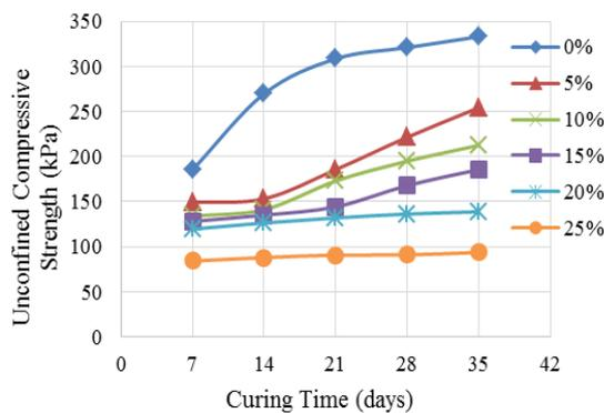
Fig. 6. Unconfined compressive strength vs. curing period
