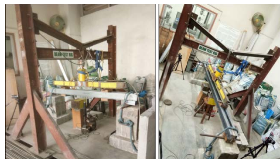
Fig.3 Actual setup of the four-point bend test
