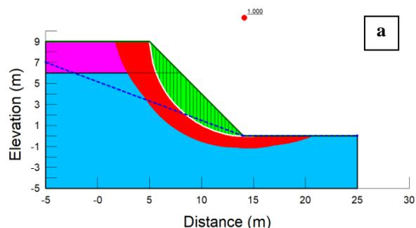
Fig.9 (a) Failure slip surface and safety map for slope model with  $H = 9m$  and  $\beta = 45^\circ$  for sample S2 (Morgenstern-Price)
