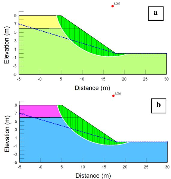
Fig.8 Failure slips surfaces for slope model with  $H = 9m$  and  $\beta = 35^\circ$  for (a) sample S1 and (b) sample S2 (Janbu)
