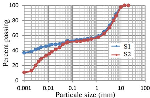
Fig.1 Grain size distribution of residual soil for samples S1 and S2
