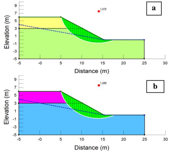
Fig.7 Failure slips surfaces for slope model with  $H = 6m$  and  $\beta = 30^\circ$  for (a) sample S1 and (b) sample S2 (Bishop)
