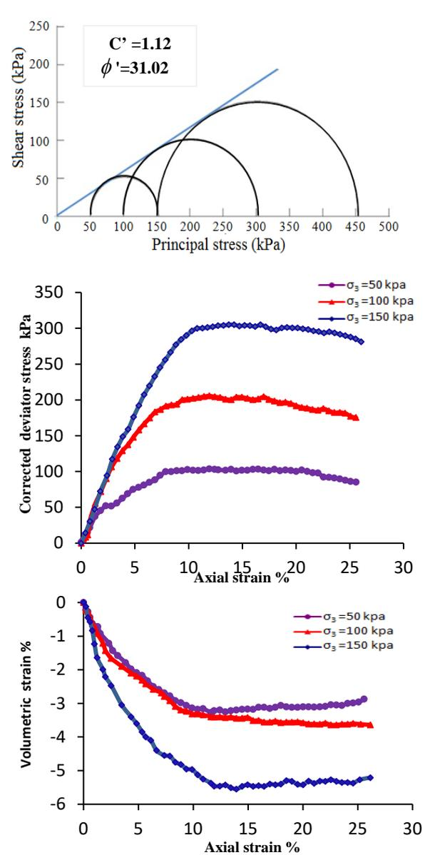
Fig. 4 Relations of effective stress failure envelope of CD test (for samples S1 that remolded with 100 kPa pressure, depth of 3.5 m), deviator stress vs. axial strain and pore water pressure vs. axial strain
