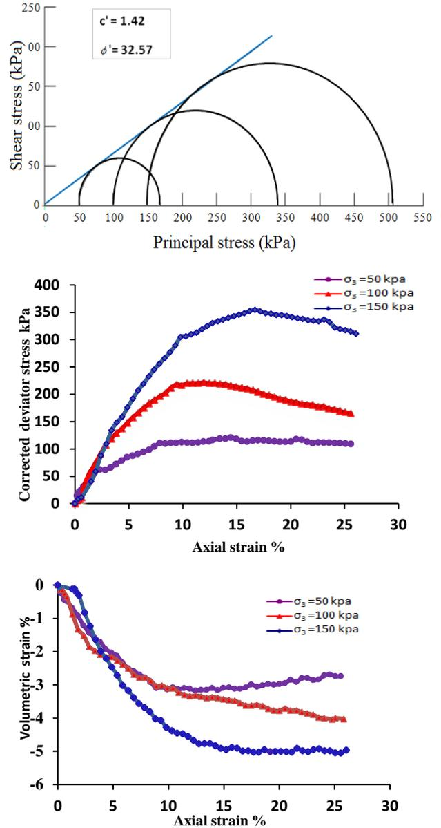
Fig. 6 Relations of effective stress failure envelope of CD test (for samples S1 that remolded with 200 kPa pressure, depth of 3.5 m), deviator stress vs. axial strain and pore water pressure vs. axial strain
