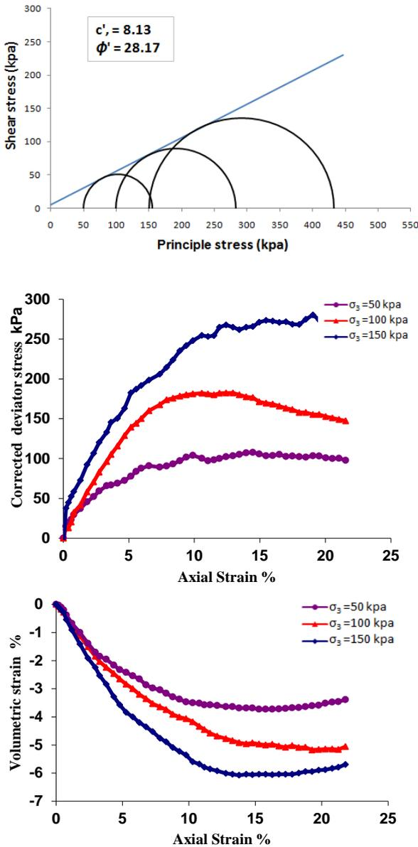
Fig. 3 Relations of effective stress failure envelope of CD test (for samples S1 that remolded with 100 kPa pressure, depth of 1.5-2.5 m), deviator stress vs. axial strain and pore water pressure vs. axial strain [5]
