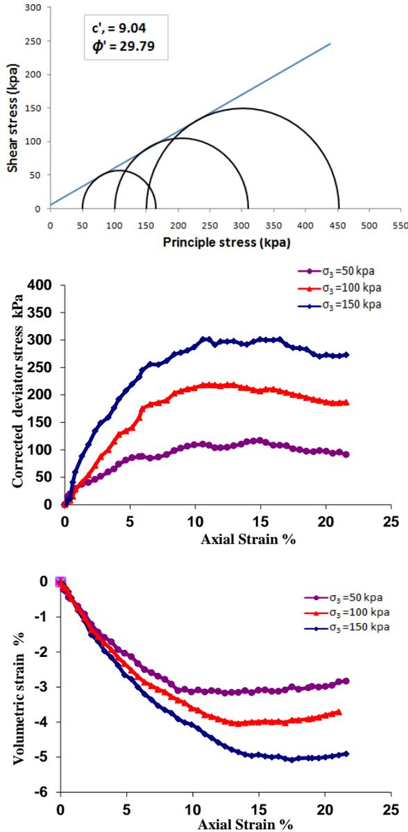
Fig. 5 Relations of effective stress failure envelope of CD test (for samples S1 that remolded with 200 kPa pressure, depth of 1.5-2.5 m), deviator stress vs. axial strain and pore water pressure vs. axial strain [5]
