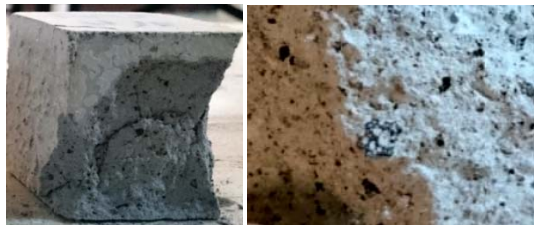
Fig.7 Failure plane of shotcrete used bottom ash as fine aggregate.
