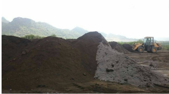
Fig.2 Landfill of bottom ash in Mae Moh mine.
