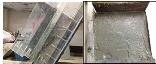
Fig. 4 Sagging and Build-up thickness of shotcrete
