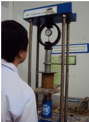
Fig. 2 The specimens conducted on unconfined compressive strength tests.
