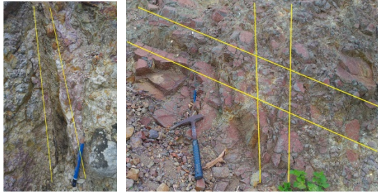
Fig. 2 Joint filled with clay minerals as mylonite at rock slopes of IM-1(left). Joint sets on platy jointed lava haze (right).
