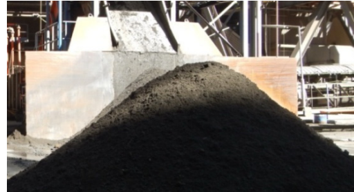
Fig.1 Bottom ash obtained from Mae Moh power plant.
