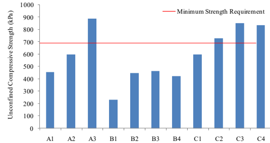
Fig. 11 The unconfined compressive strength of the soil improvement for each mixture at curing time 7 days.
