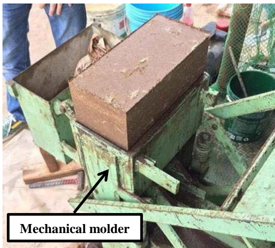
Fig.2 Photograph of the production of CEB using a mechanical molder.
