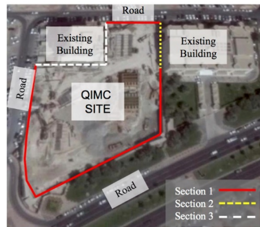
Fig. 3 Division of shoring system along the perimeter
