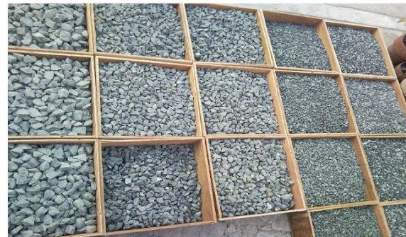
Fig. 1 Crushed coarse aggregates sizes (25mm, 19mm, 12.5mm, and 10mm)
