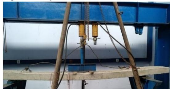
Fig. 15. Slab flexure under 4 points bending load
