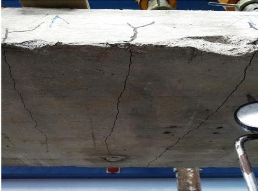
Fig. 16. Cracks on the specimen during loading test
