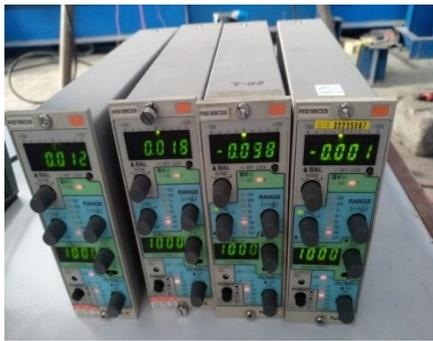
Fig. 17. Dynamic strain amplifier AS-1803
