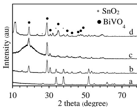
**Fig.10.** X-Ray diffraction patterns of (a) FTO and the  $\text{FTO}/\text{BiVO}_4$  prepared by the different methods of (b) Cyclic voltammetry, (c) Amperometry (d) Spin coating
