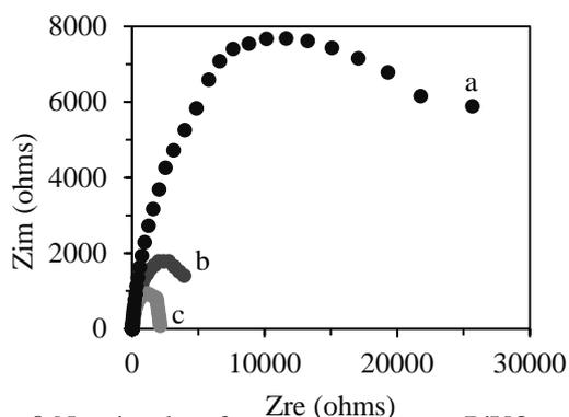
**Fig. 8** Nyquist plot of  $\text{BiVO}_4$  electrode prepared by different methods of (a) spin coating (b) amperometry (c) Cyclic voltammetry
