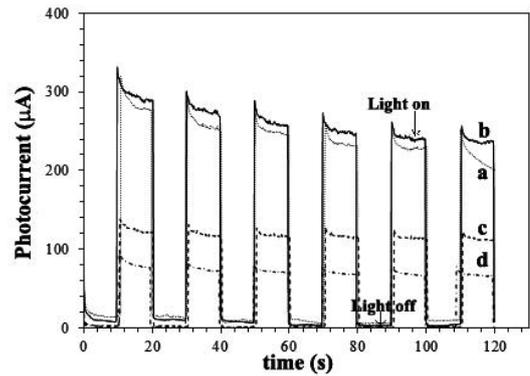
**Fig. 3.** Amperograms of FTO/BiVO<sub>4</sub> prepared by the different scan rates of (a) 25 (b) 50 (c) 100 and (d) 250 mV/s
