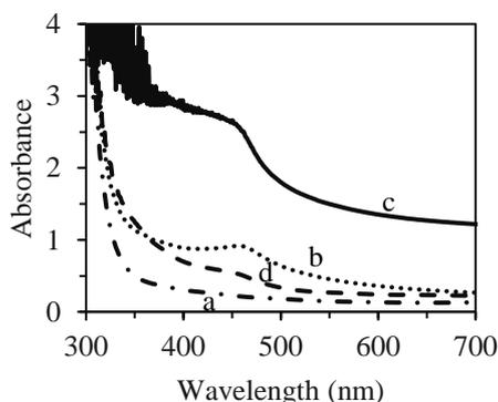
**Fig. 6.** The UV-visible spectra of (a) FTO and FTO/BiVO<sub>4</sub> electrodes prepared by different method of (b) Cyclic voltammetry (c) Amperometry and (d) spin coating
