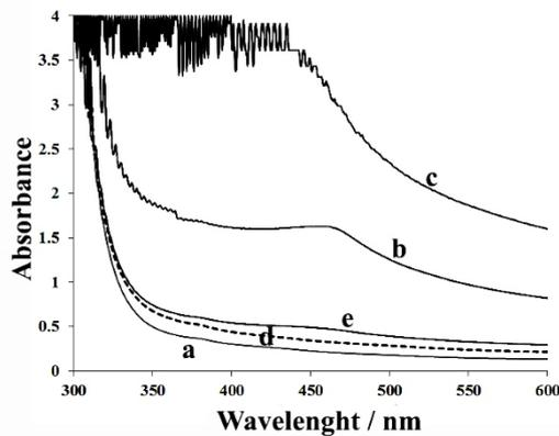
**Fig. 2.** The UV-visible spectra of (a) bare FTO and FTO/BiVO<sub>4</sub> prepared by the different scan rates of (b) 25 (c) 50 (d) 100 and (e) 250 mV/s
