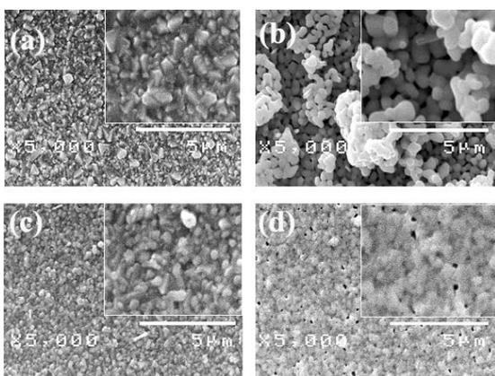
**Fig. 9.** SEM images of (a) bare FTO substrate and  $\text{FTO}/\text{BiVO}_4$  electrode prepared by the different methods of (b) Amperometry (c) Cyclic voltammetry and (d) Spin coating
