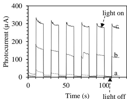
**Fig. 7.** Photocurrent of BiVO<sub>4</sub> electrode prepared by different methods (a) spin coating (b) amperometry and (c) cyclic voltammetry
