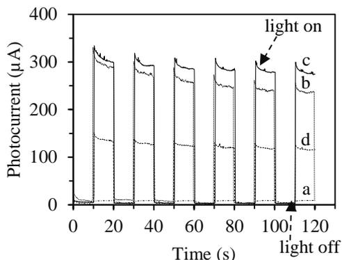
**Fig. 5.** Amperograms of FTO/ BiVO<sub>4</sub> electrode prepared by CVD method with the study of scanning cycle number (a) 1 (b) 3 (c) 5 and (d) 7 cycles
