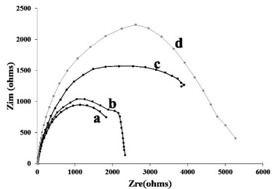
**Fig. 4.** Nyquist plot of FTO/BiVO<sub>4</sub> prepared by the different scan rates of (a) 25 (b) 50 (c) 100 and (d) 250 mV/s
