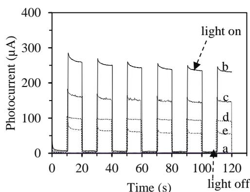
**Fig. 1.** Amperograms of FTO/BiVO<sub>4</sub> prepared with the different precursor solution temperatures of (a) Room Temperature (b) 40 °C (c) 50 °C (d) 60 °C and (e) 70 °C
