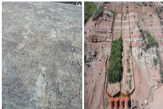
Fig. 3 Comparison of treated and control area. (a) a few cracks in the consolidation and waterproof area, (b) comparison with two plots in September in 2014
