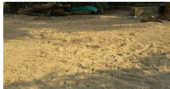
Fig. 4 Fine sand ejected through ground cracks.
