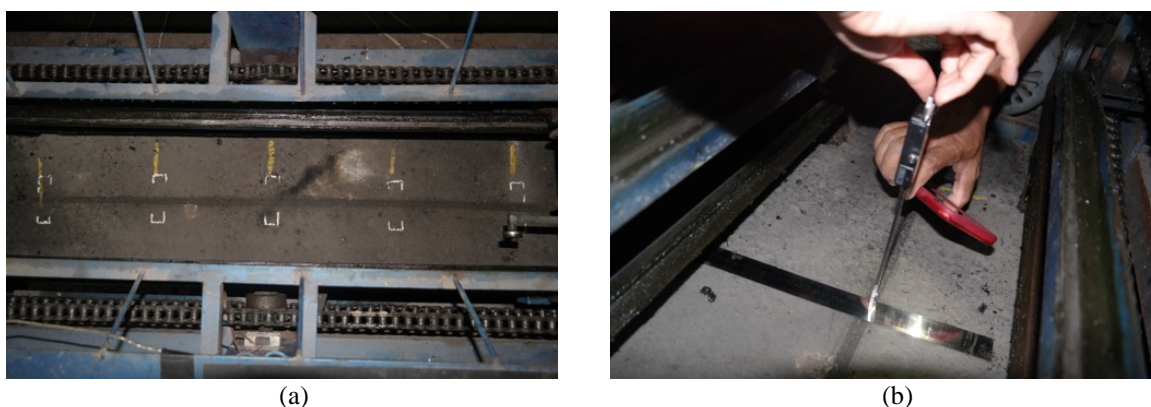
Fig. 8. Deformation measurement; (a) location of deformation measurements, (b) measurement process
