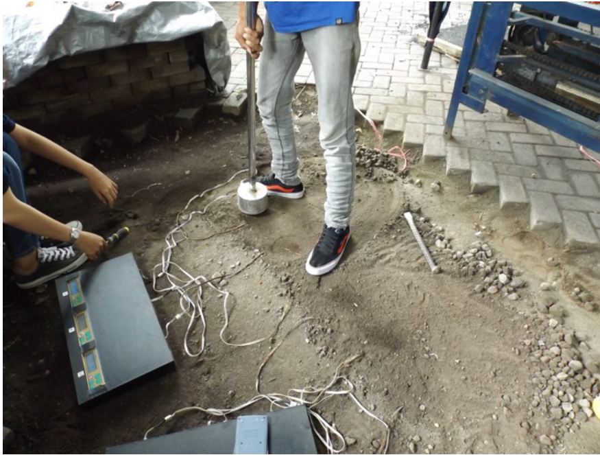
Fig. 2. Installation of strain gauges in base layer of the test section
