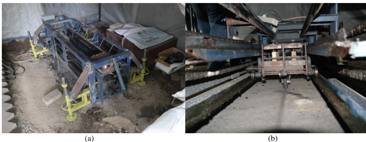
Fig. 7. Loading device used to simulate traffic loading in the test section. (a) overall view of device, (b) loading mechanism of pavement
