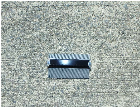
Fig. 3 Measurement surface with arithmetical mean roughness of 0.30 mm
