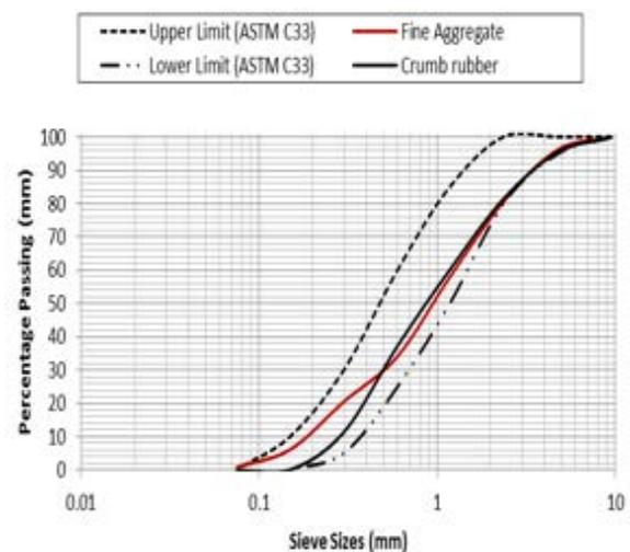
Fig. 1 Sieve analysis of aggregate
