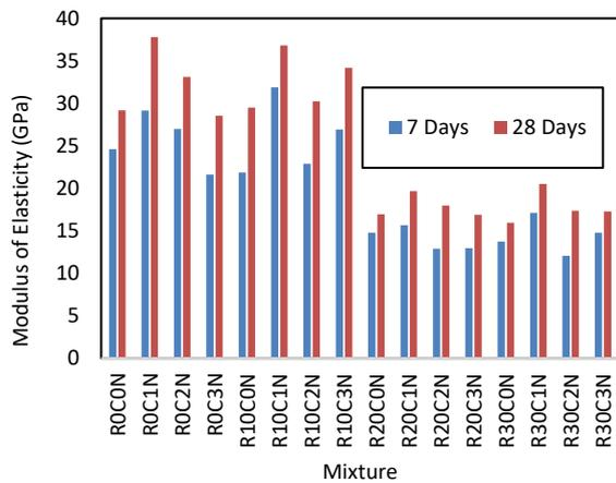
Fig. 4a Modulus of Elasticity of RCR
