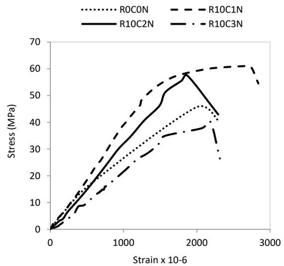
Fig. 5a Stress-strain curve for (a) RCR with 0%-10% CR
