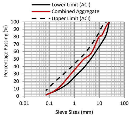
Fig. 2 Combined aggregate grading
