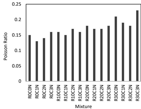
Fig. 4b Poisson's Ratio of RCR
