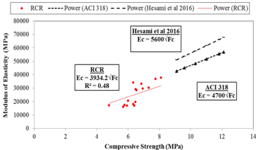
Fig. 6 Power relation between MOE and compressive strength of RCR
