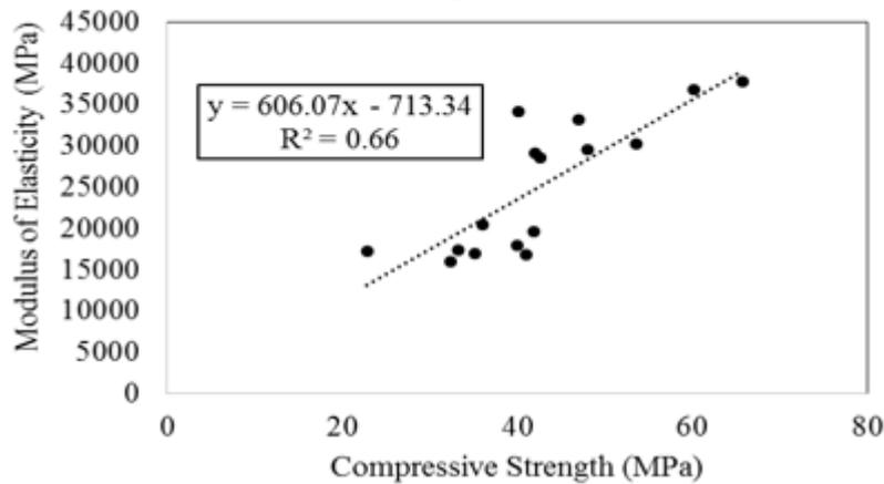
Fig. 7 Recommended relationship between MOE and compressive strength of RCR
