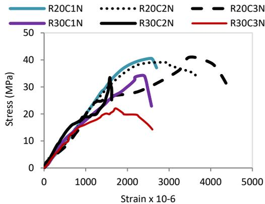
Fig. 5b Stress-strain curve for RCR with 20%-30% CR
