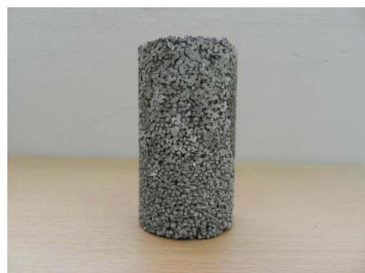
Fig. 1 Laboratory pervious concrete sample
