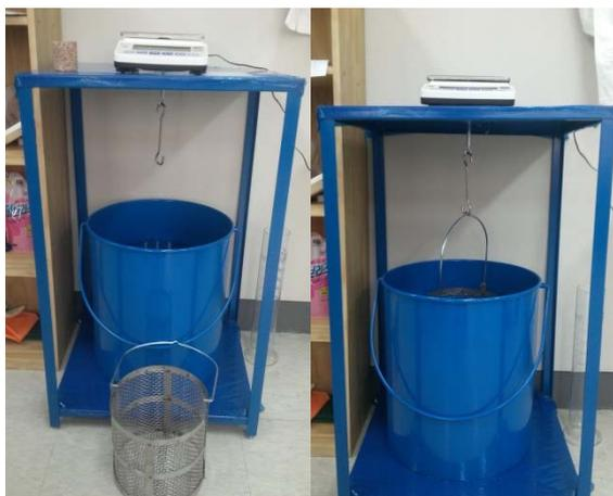
Fig. 2 Measurement of submerged weights
