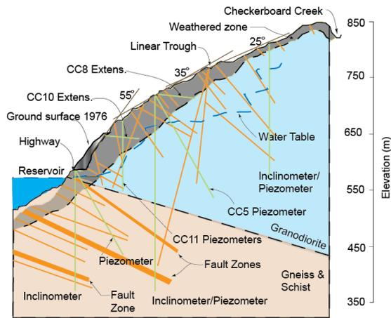
Fig. 2 Cross-section along the Checkerboard Rock Slope (modified from [7])
