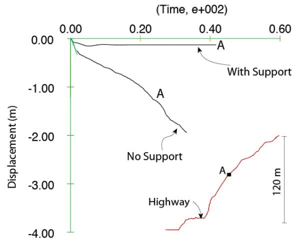
Fig.10 Effect of supporting system on the displacement of surface point A
