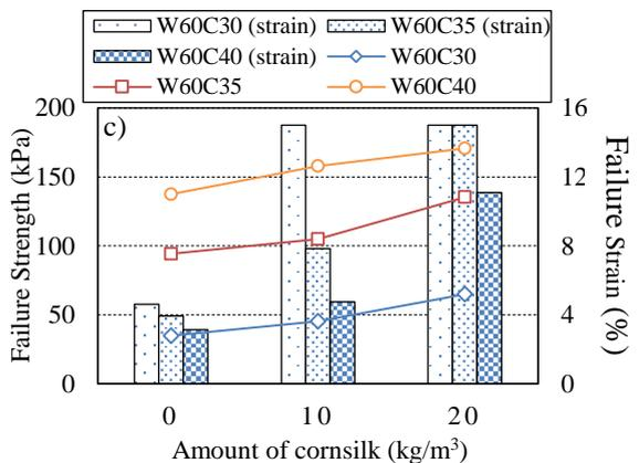
Figs.8a, 8b, 8c Relationship between failure strength and strain and additive amount of cornsilk with different additive amount of water and cement
