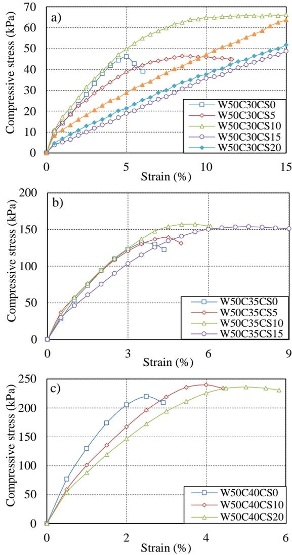
Figs.4a, 4b, 4c Stress-strain curves at water content of 50%
