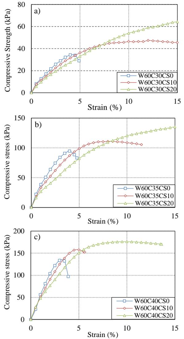
Figs.5a, 5b, 5c Stress-strain curves at water content of 60%
