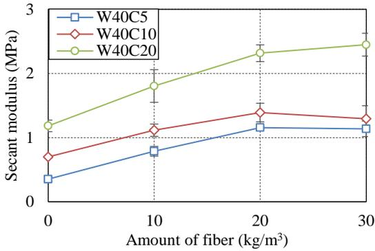
Fig. 6 Relationship between secant modulus and fiber content at strain of 2% and water of 40%
