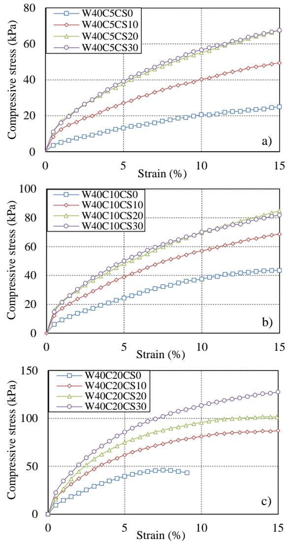
Figs.3a, 3b, 3c Stress-strain curves at water content of 40%
