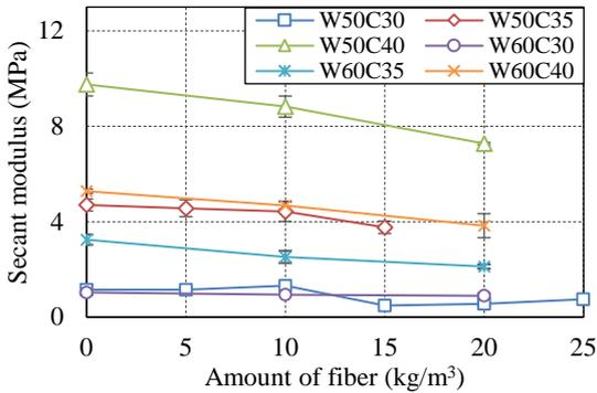
Fig.7 Relationship between secant modulus and fiber content at strain of 2% and water of 50% and 60%
