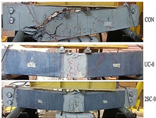
Fig.5 Failure mode of reference beams
