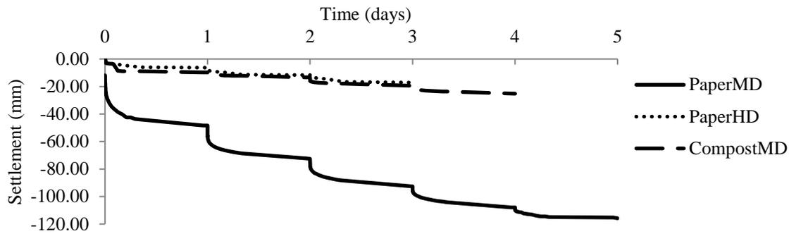
Fig. 2 The trend of the time versus settlement of Paper<sub>MD</sub>, Paper<sub>HD</sub> and Compost<sub>MD</sub>
