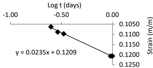
Fig. 5 Determination of  $C_\alpha$  of Paper<sub>MD</sub> at the stress of 2.05 kPa.
