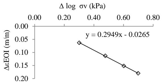
Fig. 4 Determination of  $C_c'$  on Paper<sub>MD</sub>.
