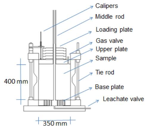
Fig. 1 Scheme of the compression cell.
