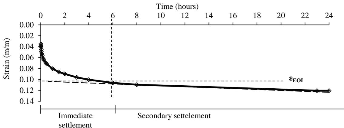
Fig. 3 Determination of  $\epsilon_{EOI}$  of Paper<sub>MD</sub> at a stress of 2.04 kPa.
