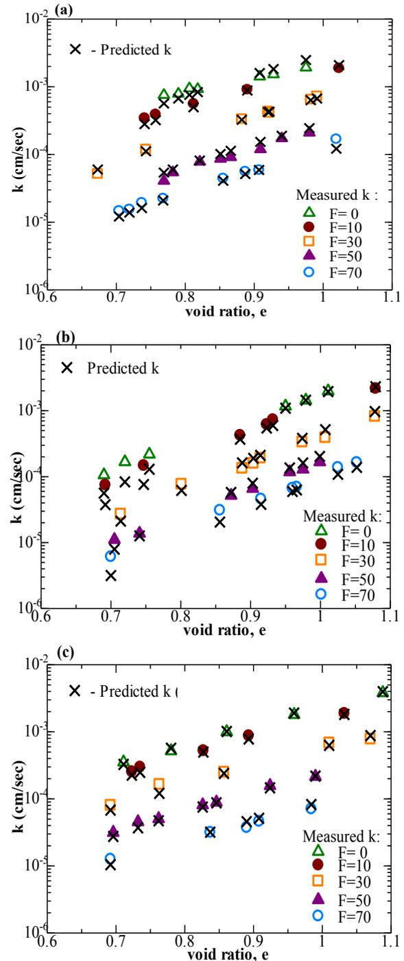
Fig. 4 Validation of the proposed equations for  $k$  (a) TS#1 (b) TS#2 and (c) TS#3
