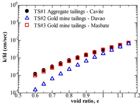
Fig. 5 Predicted  $k$  of mine tailings as function of void ratio
