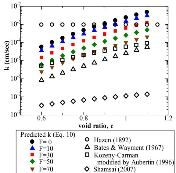
Fig. 8 Comparison of predicted  $k$  using Eq. (10) with equations from literature
