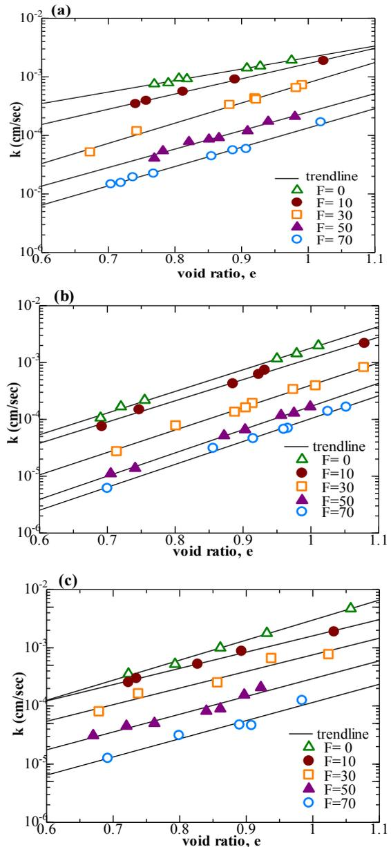
Fig. 3 Measured  $k$  vs. void ratio,  $e$  (a) TS#1 (b) TS#2 (c) TS#3
