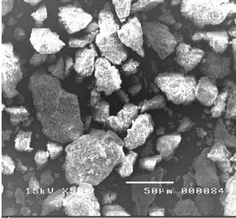
TS#1 - Wastes from aggregate quarry in Cavite
