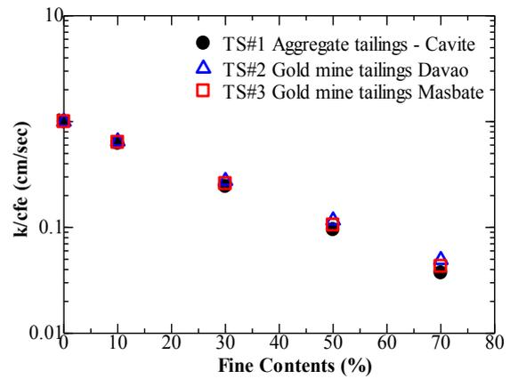
Fig. 6 Predicted  $k$  of mine tailings as a function of fine contents
