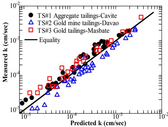
Fig. 7 Measured vs predicted  $k$  values of mine tailings
