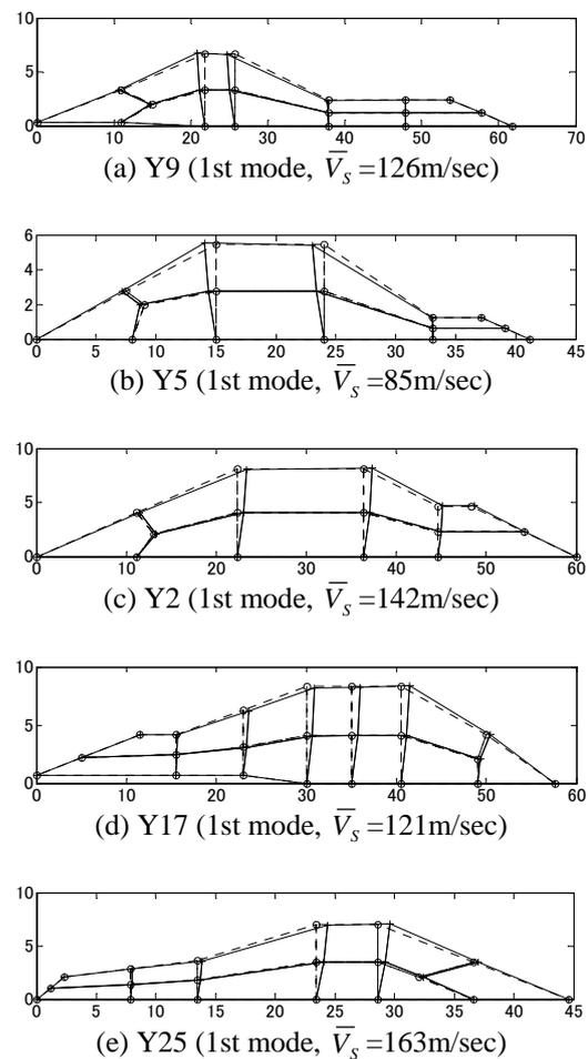
Fig.7 Identified Finite Element Model (1st mode)
