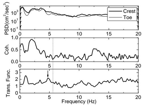
Fig.5(b) Power Spectral Density Function, Coherence Function and Transfer Function at Y5
