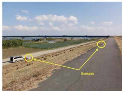
Fig.3 Microtremor measurement at levee site
