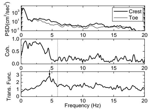
Fig.5(d) Power Spectral Density Function, Coherence Function and Transfer Function at Y17
