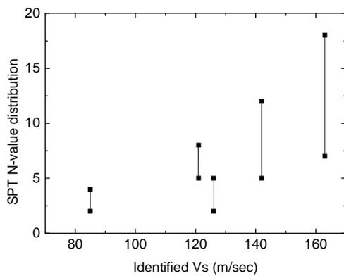
Fig. 6 SPT-N value and Identified Vs at each site
