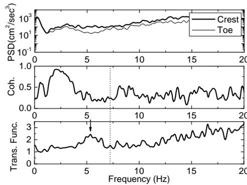
Fig.5(c) Power Spectral Density Function, Coherence Function and Transfer Function at Y2
