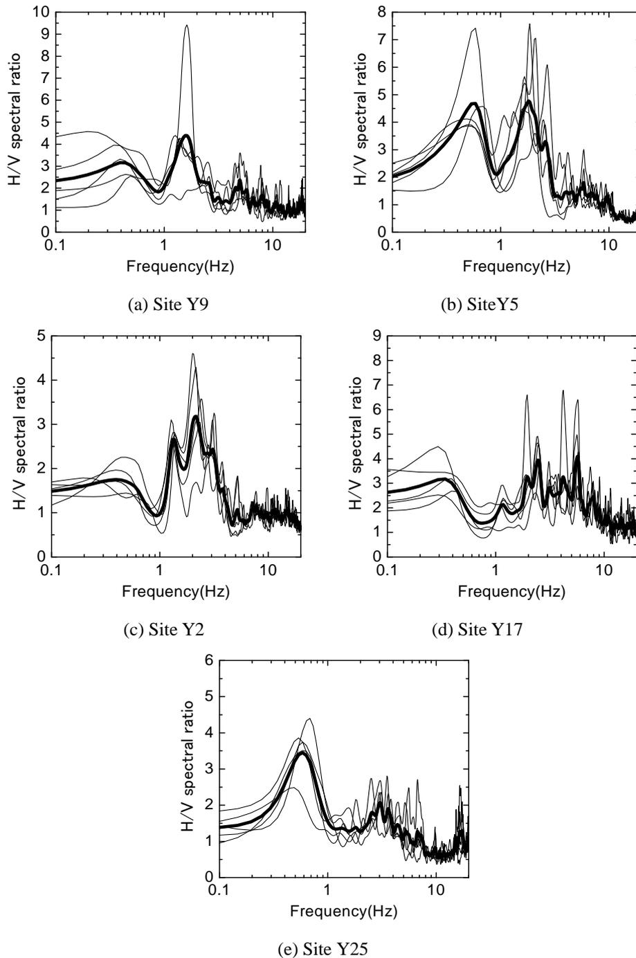
Fig.4 H/V Spectral Ratio (thick line is average of other thin lines)
