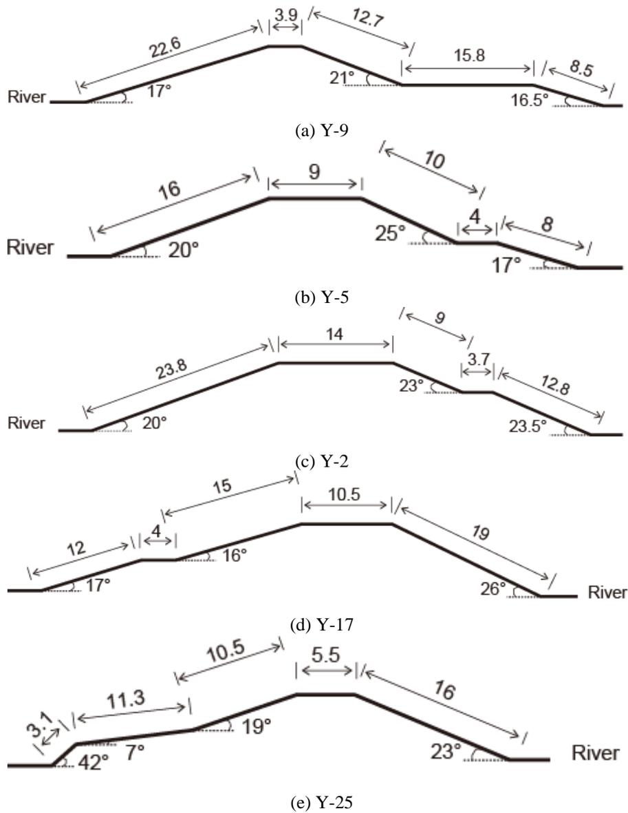
Fig.2 Cross sections of levee (unit in meters)
