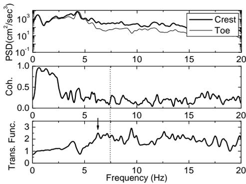
Fig.5(a) Power Spectral Density Function, Coherence Function and Transfer Function at Y9
