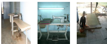
Fig. 4 The equipments used in the production Bang grass: Bang squeezer; looms; sewing machine.
