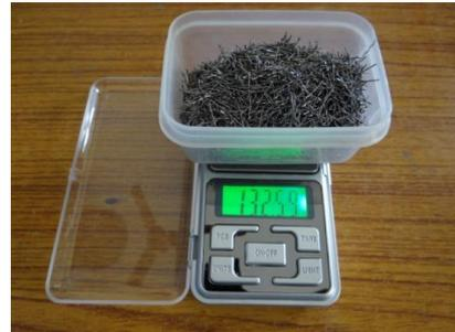
Fig. 2. Weighing the Mild Steel Fibers
