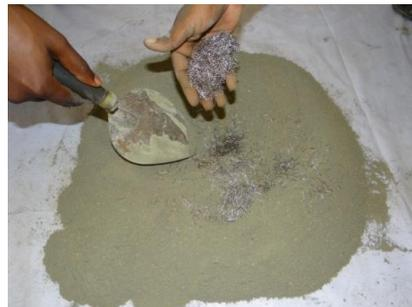
Fig. 3. Spreading MS fibers to Dry Mortar
