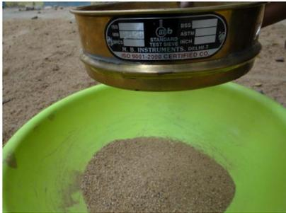
Fig. 1 Sand passing through 2.36 mm sieve
