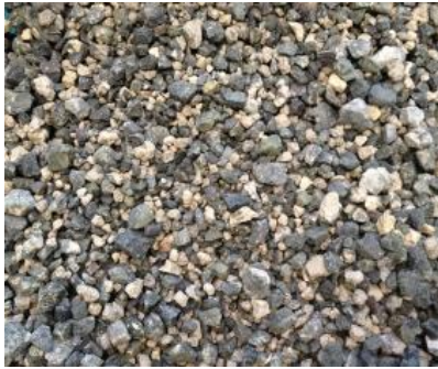
Fig. 2 Appearance of recycled aggregate concrete by pulse power discharge.
