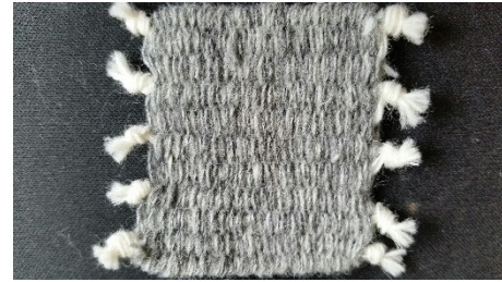
Fig. 4 Example of the proposed clad-removed POF based weave structure (plain weave)
