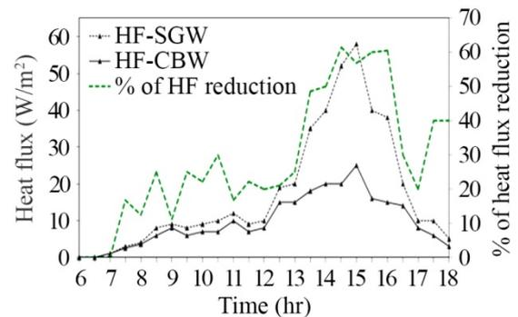
Fig.11 Hourly variations in heat flux and percentage heat flux reduction of SGW and CBW on 04/10/2020
