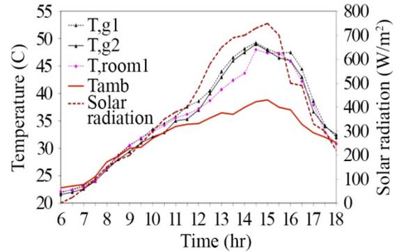
Fig.8 Temperature variations in house model H1 on 04/10/2020
