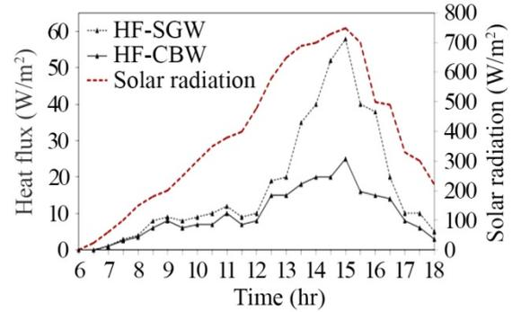
Fig.10 Hourly variations in heat flux and solar radiation of the SGW and CBW on 04/10/2020
