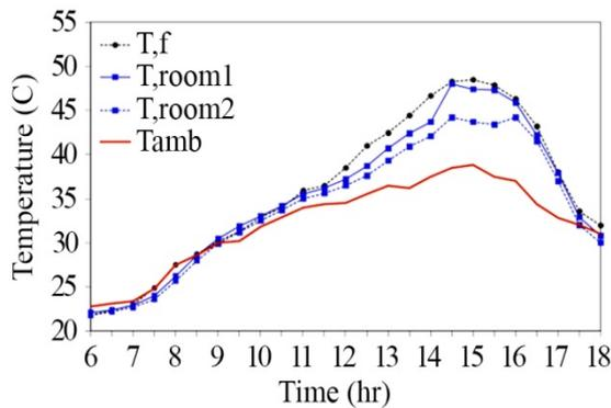
Fig.7 Comparison of room temperature variations in the house models and the clear block wall air gap temperature on 04/10/2020
