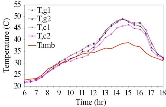
Fig.6 Comparison of the surface temperature of the single glass wall and clear block wall on 04/10/2020
