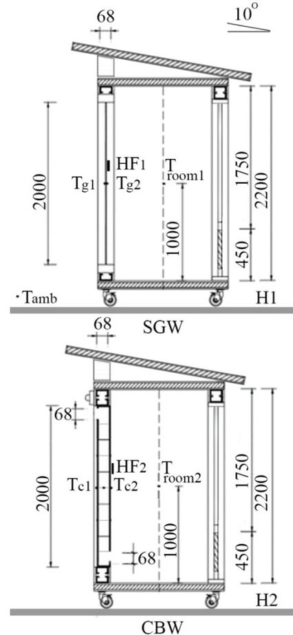
Fig.5 Detector positions outside and inside the house models
