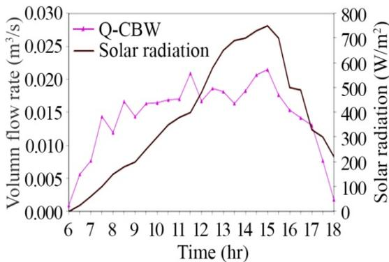
Fig.12 Hourly variations in the volume flow rate and solar radiation of the CBW on 04/10/2020
