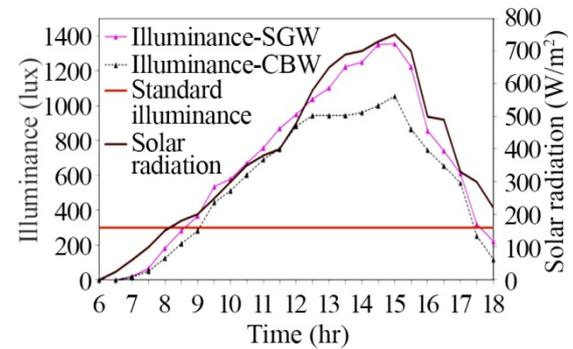
Fig.14 Hourly variations in illuminance and solar radiation of the SGW and CBW on 04/10/2020
