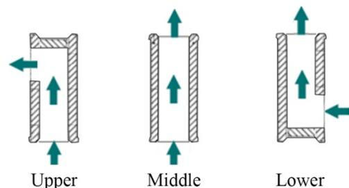
Fig.3 Cavity between the blocks to allow stack airflow
