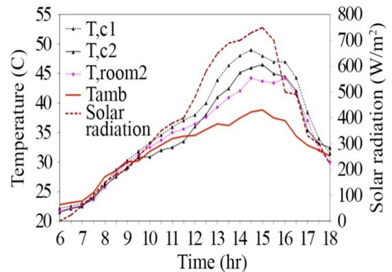
Fig.9 Temperature variations in house model H2 on 04/10/2020
