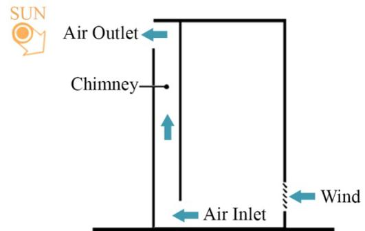
Fig.2 Solar chimney diagram
