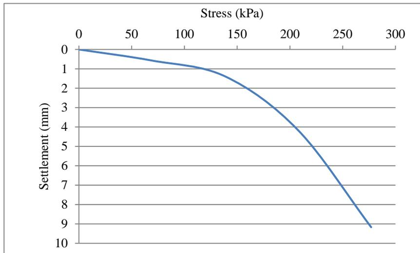
Fig. 6 Pressure-settlement curve
