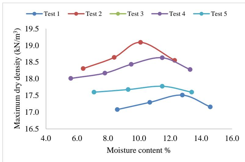
Fig. 5 Compaction curves for soil different samples
