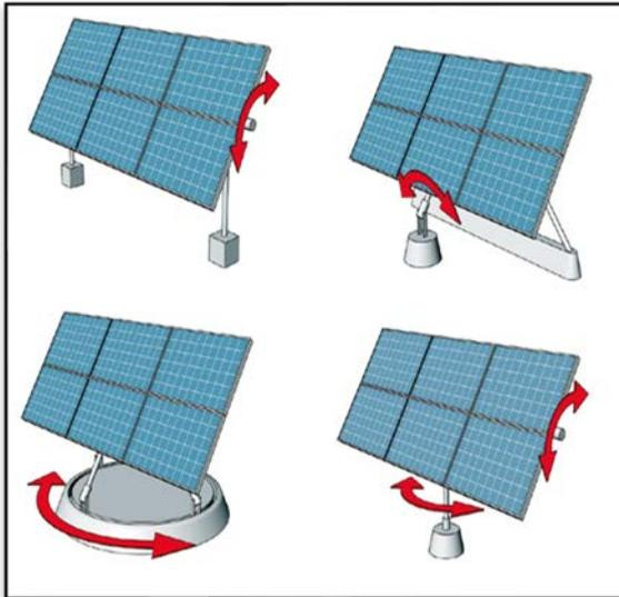
Fig. 1 Different tracking systems [5], [23]
