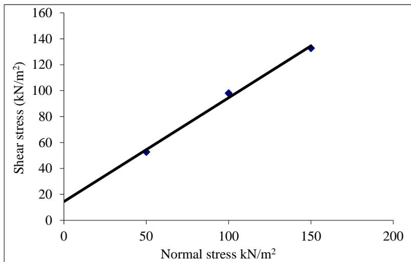
Fig. 4 Normal stress versus shear stress
