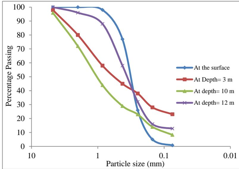
Fig. 3 Grain size distribution curves
