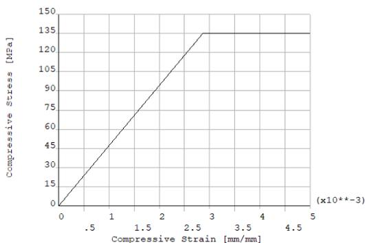
Fig.4 Compressive stress-strain for UHPFRC
