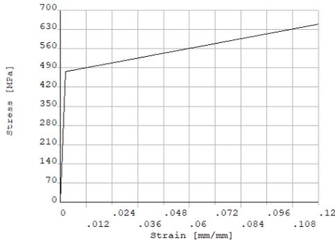
Fig.2 Stress-strain relationship for reinforcing steel
