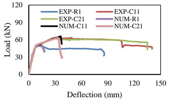
Fig.8 FE and Experimental Results (R1-C11-C21)
