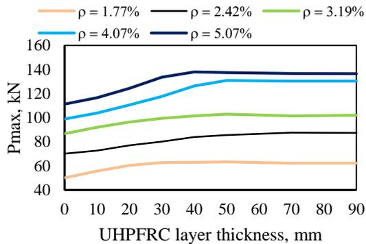
Fig.19 Effect of the thickness of UHPFRC layer and the tensile reinforcement ratio on the peak load
