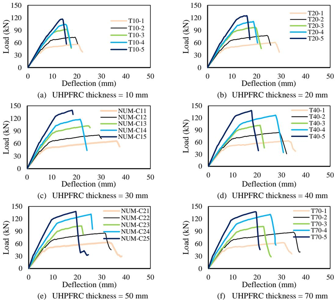
Fig.18 Load-deflection curves at mid of span at various thicknesses of UHPFRC layer (FE models)
