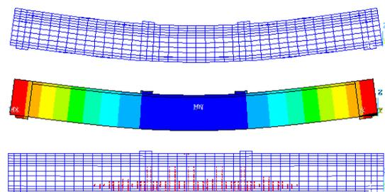
Fig.16 Deformed shape and crack pattern
