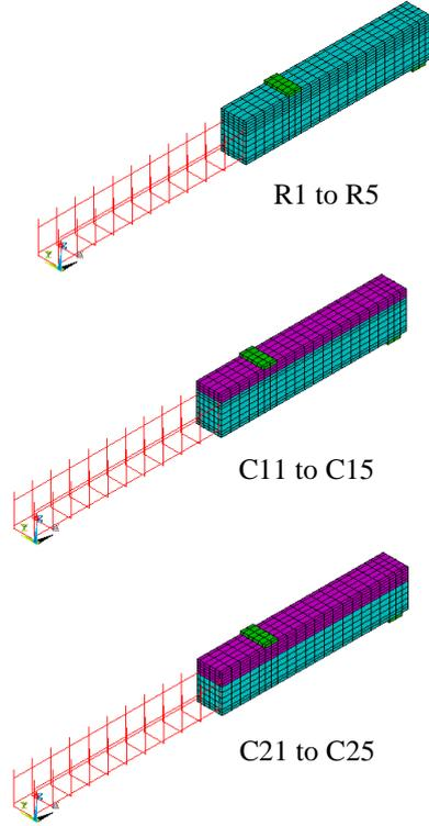
Fig.6 Finite element mesh, composite beams
