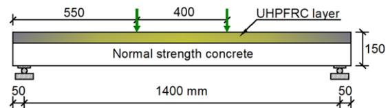
Fig.5 Geometry, loading, and beam dimensions
