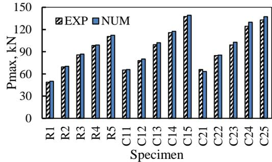
Fig.15 FE and Experimental Results ( $P_{max}$ )
