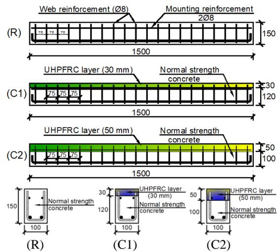
Fig.1 Details of the modeled composite beams (all dimensions are in mm)
