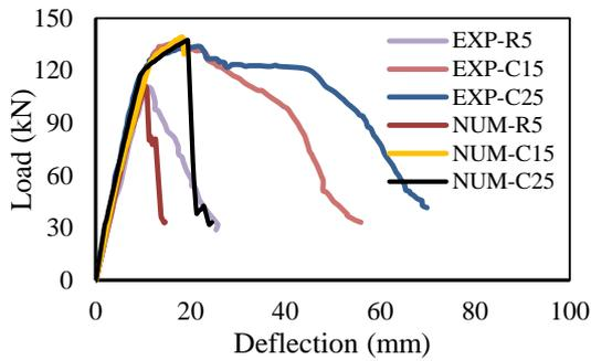
Fig.12 FE and Experimental Results (R5-C15-C25)
