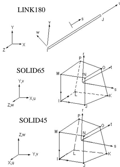
Fig.7 Geometry of elements (FE model)
