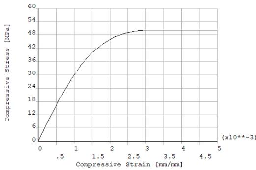
Fig.3 Compressive stress-strain relationship for concrete
