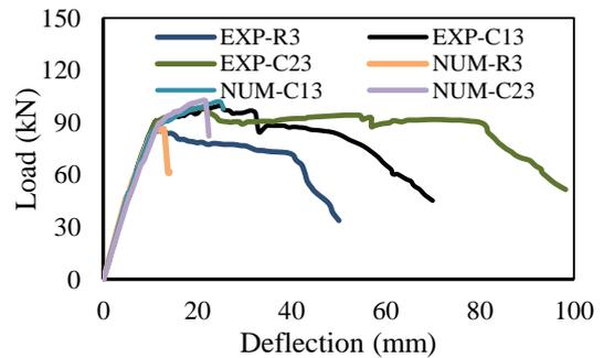
Fig.10 FE and Experimental Results (R3-C13-C23)
