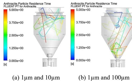
Fig. 7 The path of interested particle sizes
