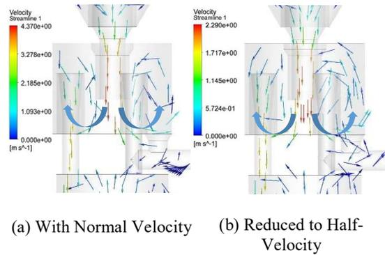
Fig. 6 Velocity streamlines in the separation chamber
