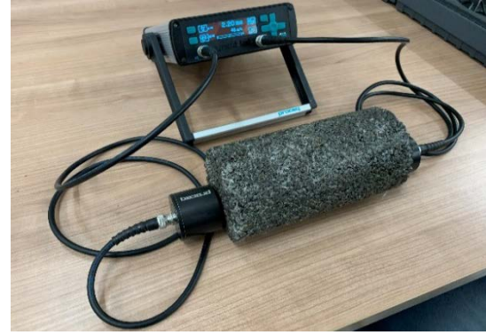
Fig.3 Ultrasonic pulse velocity (UPV) test
