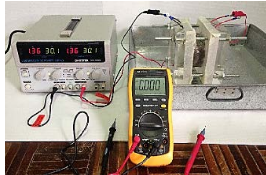
Fig.4 Chloride Penetration Test Apparatus
