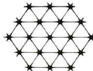
Fig. 5: Tensar TriAx Geogrid layer.
