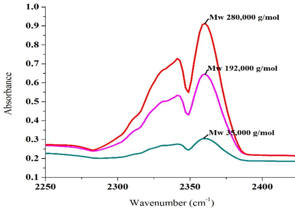
Fig. 4 The FTIR nitrile spectra of the polystyrene surface treated by nitrogen plasma with different Mw
