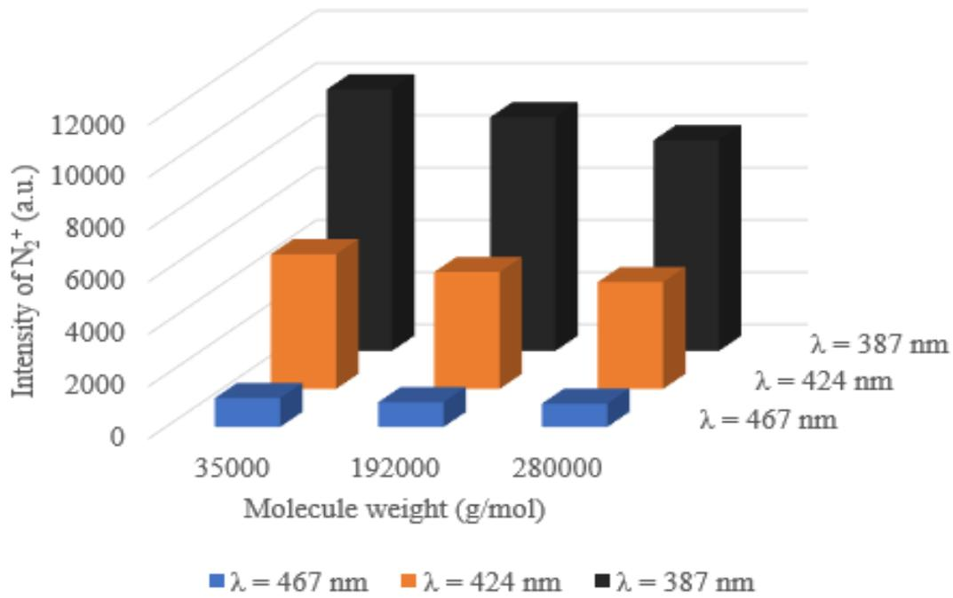
Fig 3. The OES intensity of emission spectral ion N<sub>2</sub><sup>+</sup> in the polystyrene surfaces during plasma process with different Mw
