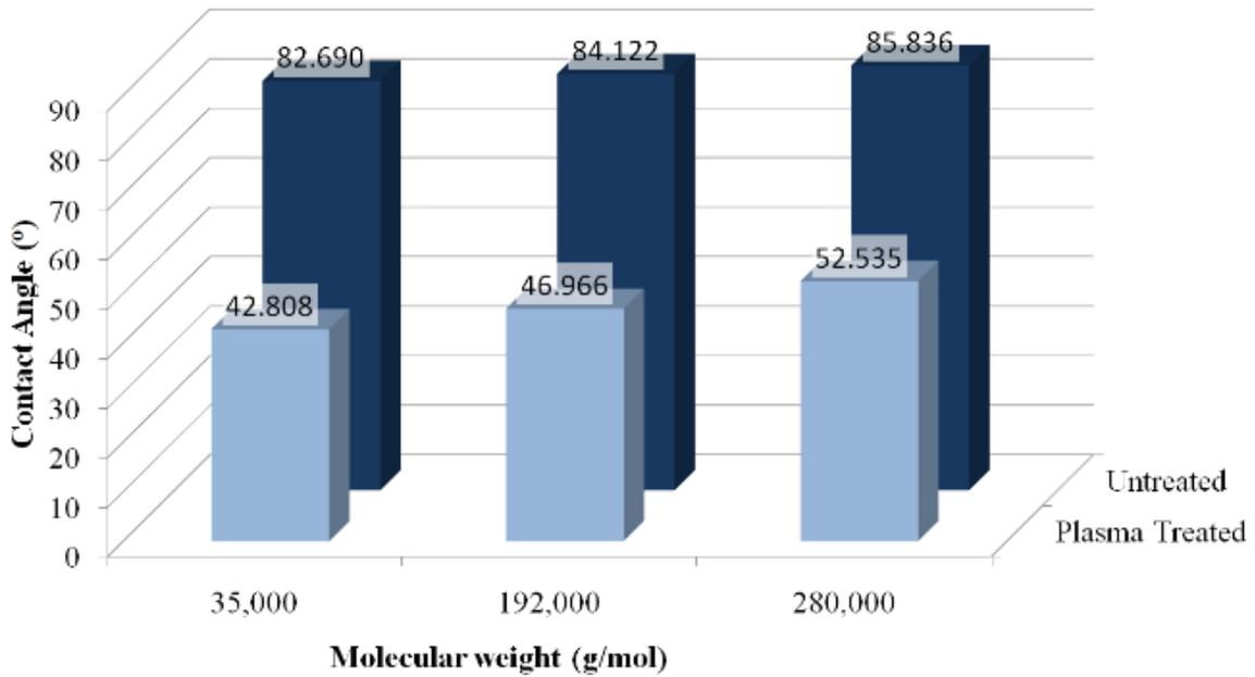
Fig. 5 The effect of various Mw on the hydrophobicity of the polystyrene surface before and after plasma treatment
