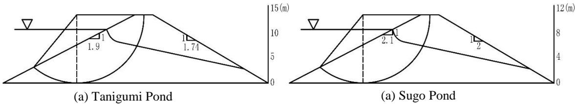
Fig.5 Schematic diagram of irrigation tanks and slip circles
