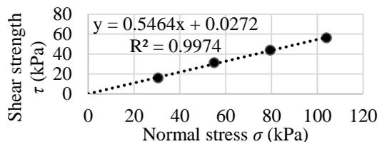
Fig.2 Shear strength vs. horizontal displacement and shear strength envelope in Tanigumi Pond soil (US)
