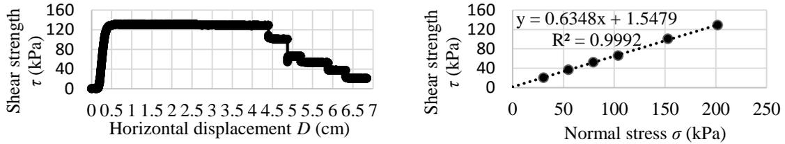
Fig.3 Shear strength vs. horizontal displacement and shear strength envelope in Sugo Pond soil (S)
