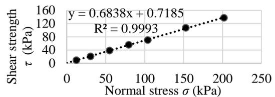
Fig.1 Shear strength vs. horizontal displacement and shear strength envelope in Tanigumi Pond soil (S)
