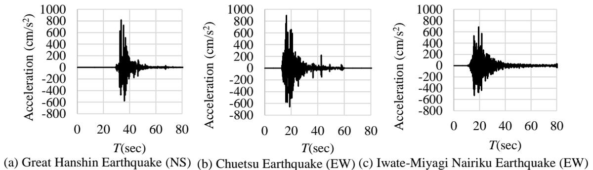
Fig.6 Input acceleration
