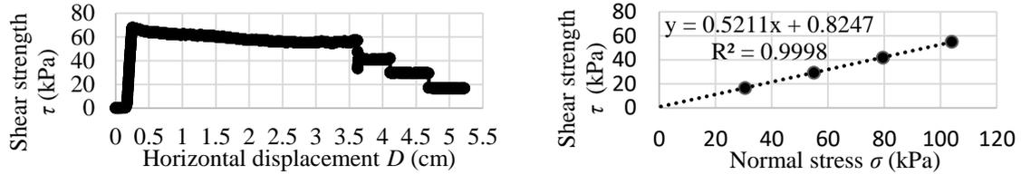
Fig.4 Shear strength vs. horizontal displacement and shear strength envelope in Sugo Pond soil (US)
