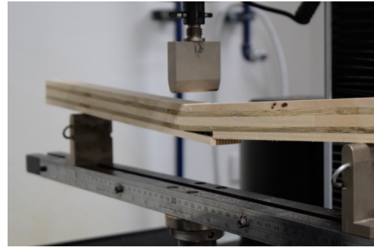
Fig. 7 The fracture at the tension tie of 2" x 4" Glued Bamboo laminated timber with Para-timber [9]
