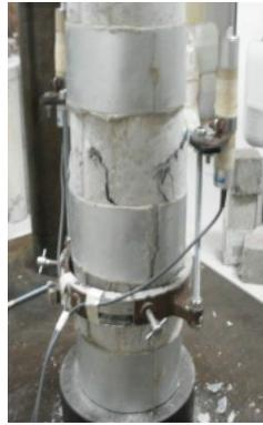
Fig. 9 Failure of the partially confined column with metal sheet strips (C-4-12.5).
