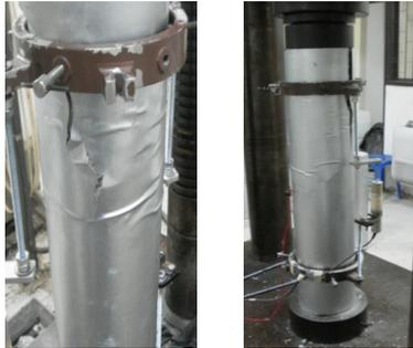
Fig. 4 Failure of the column confined with a one-piece full-wrap metal sheet (B-1-75).
