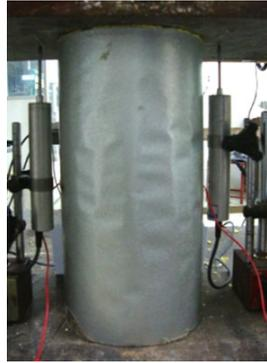
Fig. 1 Wrinkle of a metal sheet for fully wrapped confined concrete.
