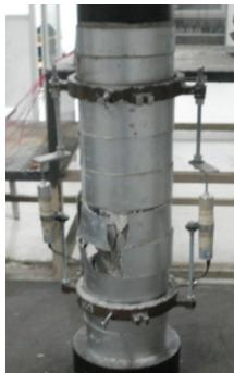
Fig. 5 Failure of the column discretely confined (C-10-7.5) with metal sheet strips.
