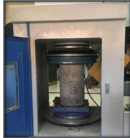
Fig. 7 Compressive test on cylindrical specimen
