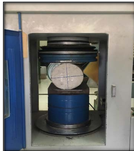
Fig. 8 Splitting tensile test on cylindrical specimen
