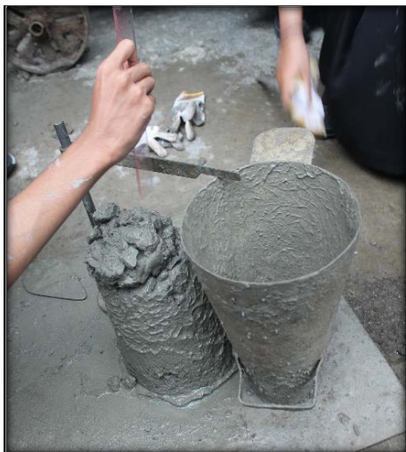
Fig. 6 Slump test on the concrete mixtures
