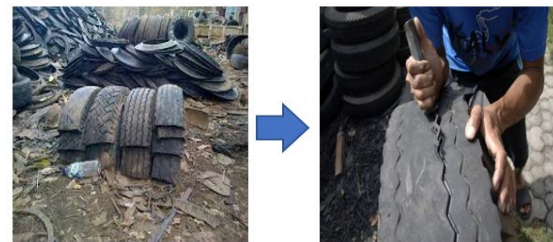
Fig. 2 Cutting process of waste tyre
