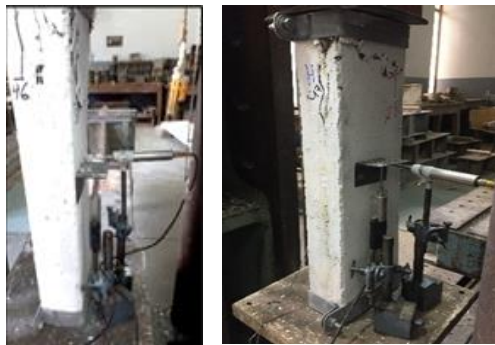
Fig.5 LVDTs locations on specimens
