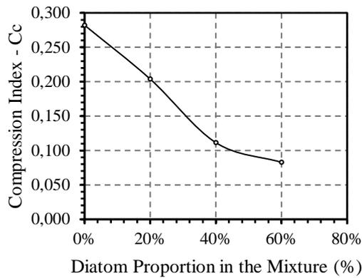
Fig. 6: Compression index of the tested samples
