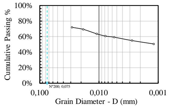
Fig. 3 Diatom particle size distribution
