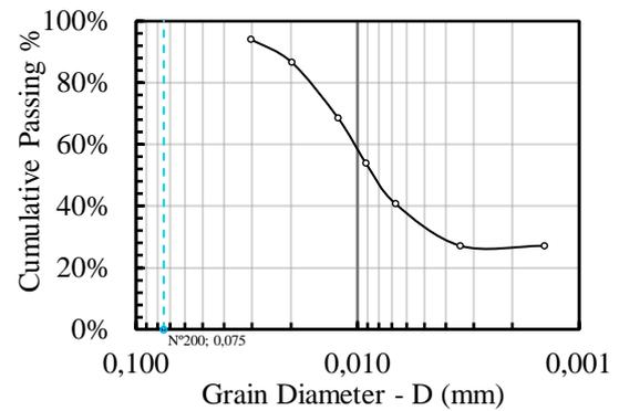
Fig. 2 Fine-grained soil particle size distribution
