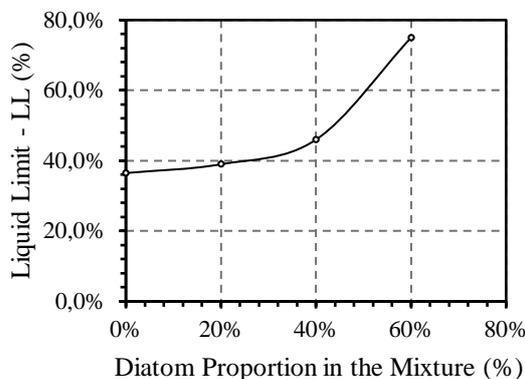
Fig. 4: Liquid limits of the tested samples
