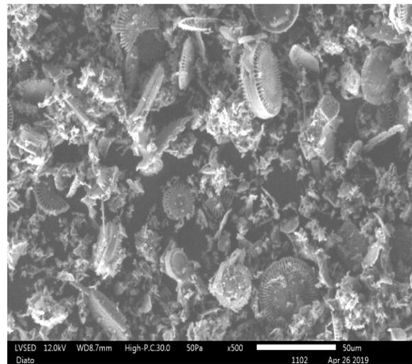
Fig. 1 Scanning electron microscopy (SEM) image of *Cyclotella Distinguenda* tested diatoms
