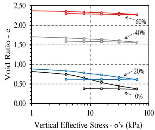
Fig. 5: Consolidation curves of tested samples
