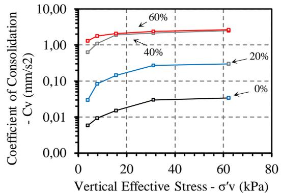
Fig 9: Coefficient of consolidation of tested samples
