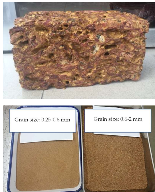
Fig.1 Laterite block (Thach That district, Hanoi, Vietnam), and crushed sieved grains
