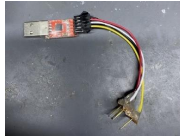
Fig. 6 USB TTL programmer adapted for series programming
