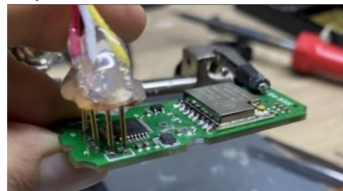
Fig. 7 Uploading software to the WMS via USB TTL programmer
