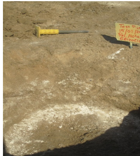
Fig.2 Sabkha soil excavation pit showing salts concentrations.
