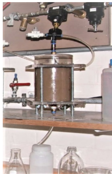
Fig.3 Experimental setup for the leaching test
